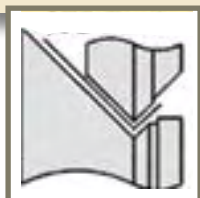
Step 1 Metal is formed 90°
